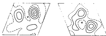
Fig. 1. Sections of an early difference map in the planes of (left) the C(9) and (right) the C(8) methyl hydrogen atoms. Contours are drawn at intervals of 0.05 e.\text{\AA}^{-3} with the zero contour dashed.
